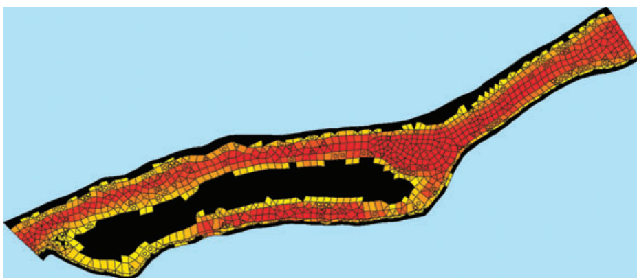
FIG. 1. The Green River study site, as depicted in the model. The site is 1000 m in length along its thalweg and depicted as 2204 polygonal cells, though some cells (■) are dry at typical flows. Cells are shaded by velocity, with redder cells faster. Each cell also has variables that represent its depth, area of velocity shelter for drift feeding and availability of hiding cover. Circles in a cell indicate the presence of one or more fishes.
